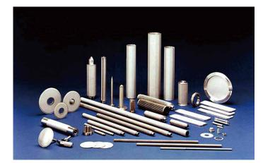
FUJIPLATE filter elements are ideal type surface filtration elements made up of several laminated layers of various alloys including stainless steel mesh sintered together to form an integrated (porous) element. A very fine gauge metal mesh with accurately controlled pore size is assembled and manufactured with protective layers and reinforcement (support) layers matched to specific
